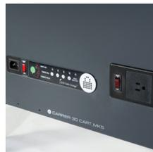
**External Charging Status Display.** Most of us don't have x-ray vision—but with our Carrier Carts, it's super easy to know the charging status of your devices through the external ECO Safe Charge™ display.
